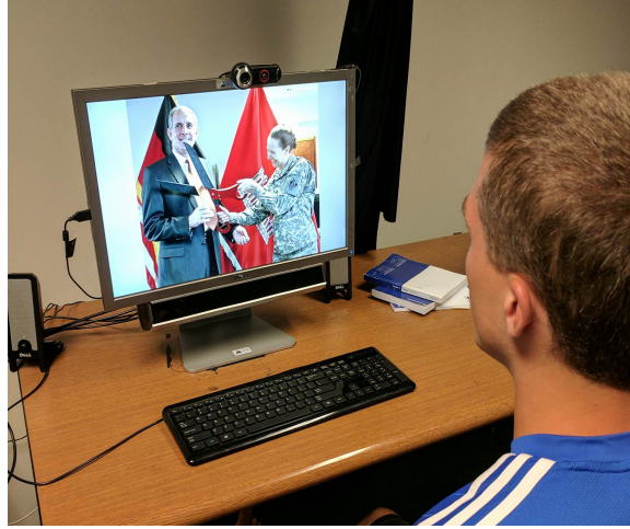
Figure 4.2: Data collection set-up used for the SNAG dataset experiment. The SMI eye-tracker that records the gaze data is attached underneath a display that displays the stimuli. The participant wears a lapel microphone connected to a TASCAM recorder that records the spoken descriptions. The task requires the participant to describe the action in the image to the experimenter.
